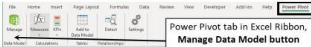
Figure 18.81 To view the Data Model, you can use the Manage Data Model button in the Excel app Power Pivot tab.
